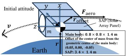
The satellite's initial attitude aligns the optical axis with the velocity vector, while rotating around it to keep the solar array panels facing the Sun—minimizing drag and torque, and maximizing power generation.
